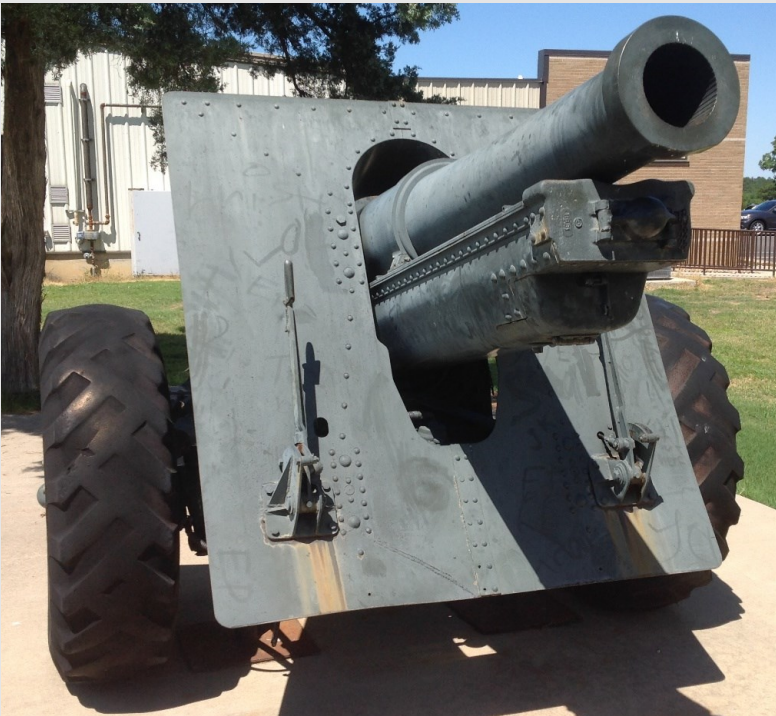
The museum's 155mm C M1917 with M1918A3 upgrades. Note the flat front plate and pneumatic tires were post WWI upgrades.
