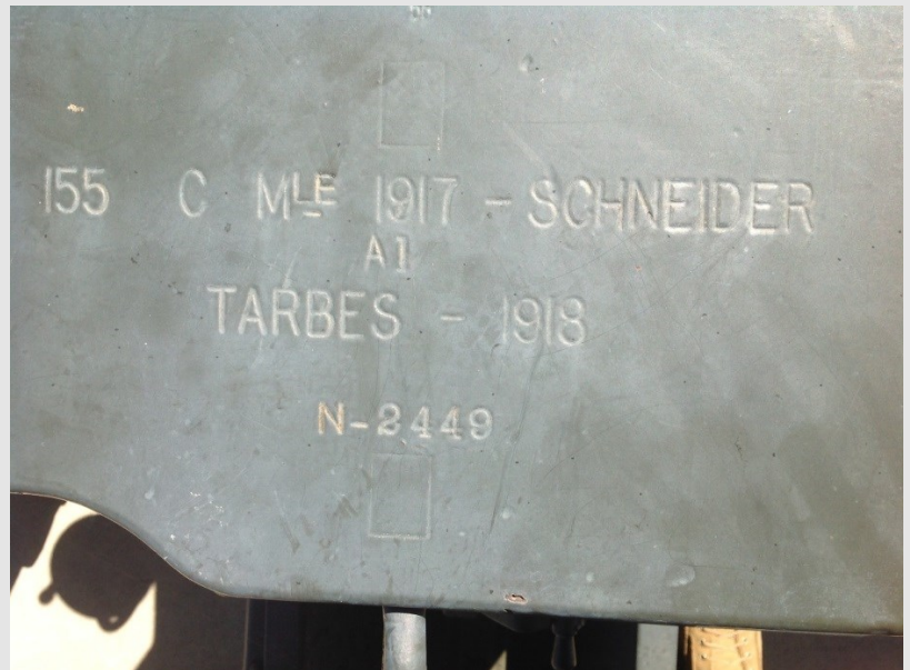
Top of Breech marked "155 C MLE 1917 - SCHNEIDER A1 TARBES - 1918 N-2449" indicating that this is a 155mm short barreled Model 1917 - Schneider which was at some point up graded and stamped A1. It was assembled in Tarbes, France in 1918 as Serial Number 2449.
