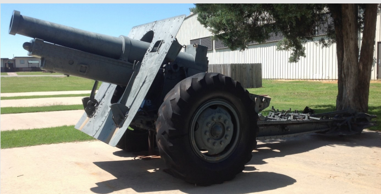
The museum's 155mm C M1917 with M1918A3 upgrades. Note the flat front plate and pneumatic tires were post WWI upgrades.
