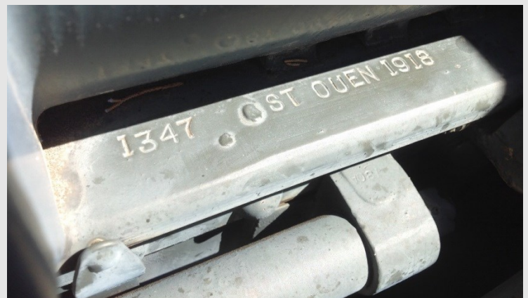
Stampings in the two photos above indicate that the some or all of the parts of the mount were made in Saint Ouen, France in 1918. 1347 indicates that it is the 1,347 th mount made.
