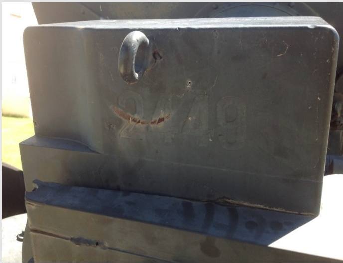
Back of the breech block is the serial number 2449, which indicates that this is the 2,449 th M1917 Schneider out of the 3,020 made in France before the Armistice.
