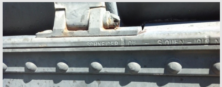
Top of Breech marked "155 C MLE 1917 - SCHNEIDER A1 TARBES - 1918 N-2449" indicating that this is a 155mm short barreled Model 1917 - Schneider which was at some point up graded and stamped A1. It was assembled in Tarbes, France in 1918 as Serial Number 2449.
