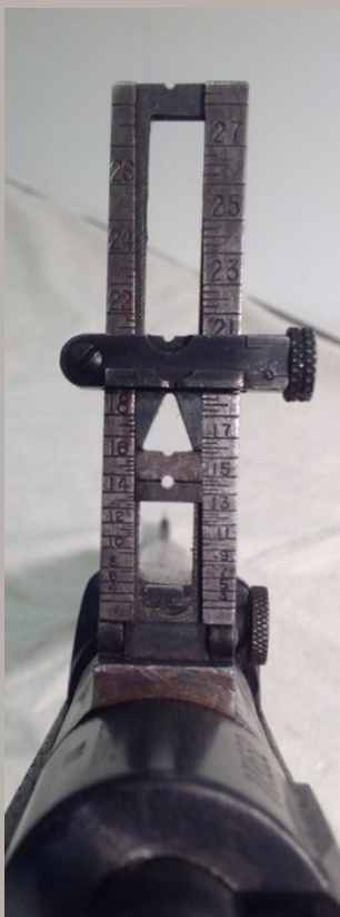
Rear sight on M1903 Springfield graduated out to 2,850 yards. Long lines represent 100 yards, medium length represent 50 yards and short lines represent 25 yards.
