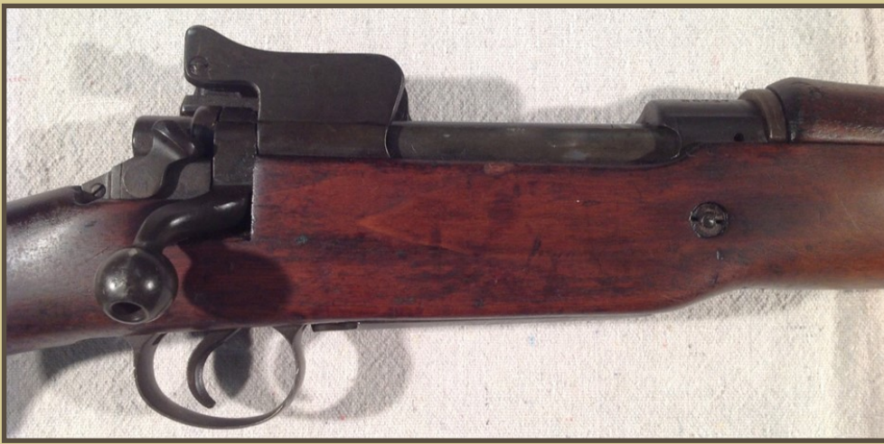
Right: Shows bolt is open position and safety switch located above the trigger. The safety could be operated silently.
