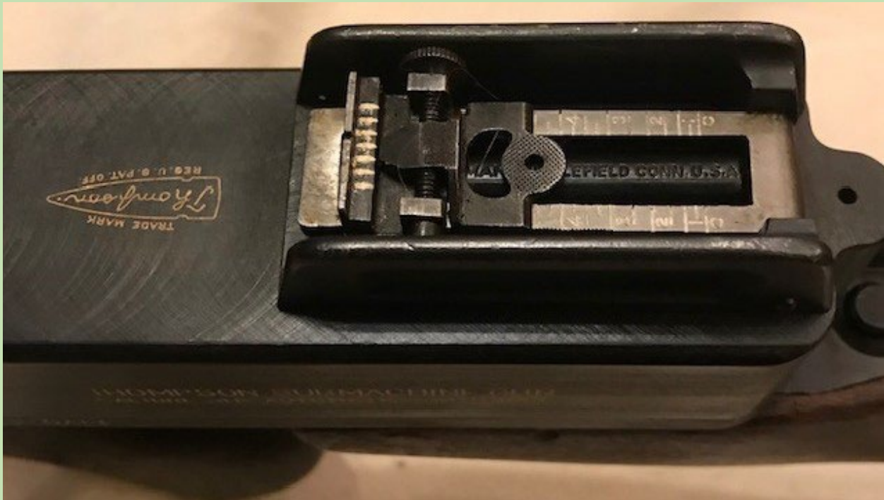
Figure 6: Complex Lyman Adjustable Rear Sight would be deemed unnecessary and replaced with an L type fixed sight to reduce cost and speed production) - Private Collection
