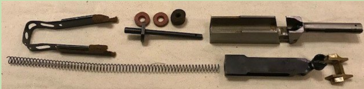
Figure 2: (Internal parts of a M1928A1. Parts remained basically unchanged in design from the Model 1919 through M1928A1. Parts shown are the U-Shaped Oiler, Buffers, Guide Rod, Spring, Lower Bolt, Upper Bolt with Charging Handle and Bronze Blish Lock, The Blish Lock slides up and down at an angle in the Lower Bolt section, grooves inside the receiver also guide the Blish Lock up and down as the bolt is blown back) – Private Collection
