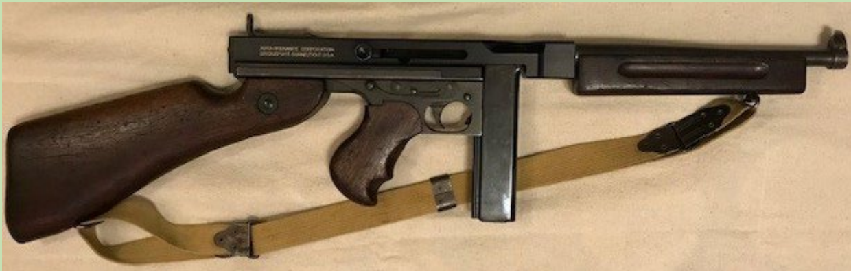
Figure 8: (M1 TSMG – Note stock is not removable, simplified rear L sight, charging handle on right side, no Cutts compensator) – Private collection
