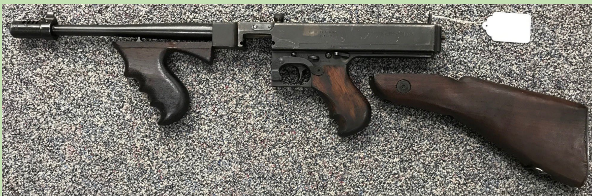
Figure 11: Note the detachable stock. Also note simplified rear L type sight, smooth tapered barrel without fins indicating the measures taken to simplify production. It is likely that the forward grips were spares that law enforcement possibly requested be added since they are not consistent with late production M1928A1s
