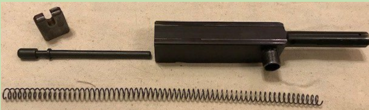
Figure 9: M1 TSMG Bolt, Spring, Guide Rod and Buffer. Note bolt handle is now on the side. This bolt would be further simplified by removing the floating spring and firing pin and machining a fixed firing pin head to the face of the bolt in the M1A1 – Private Collection
