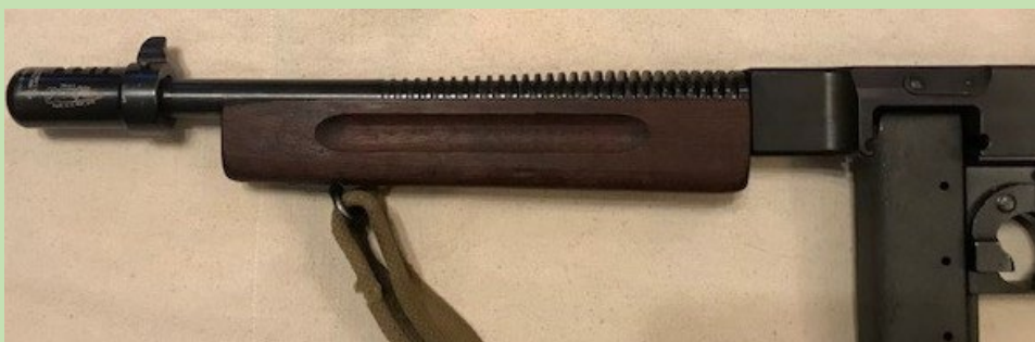
Figure 7: (Finned barrel with Cutts Compensator and horizontal fore grip as found on Lend Lease and early wartime production M1928A1 TSMG) – Private Collection
