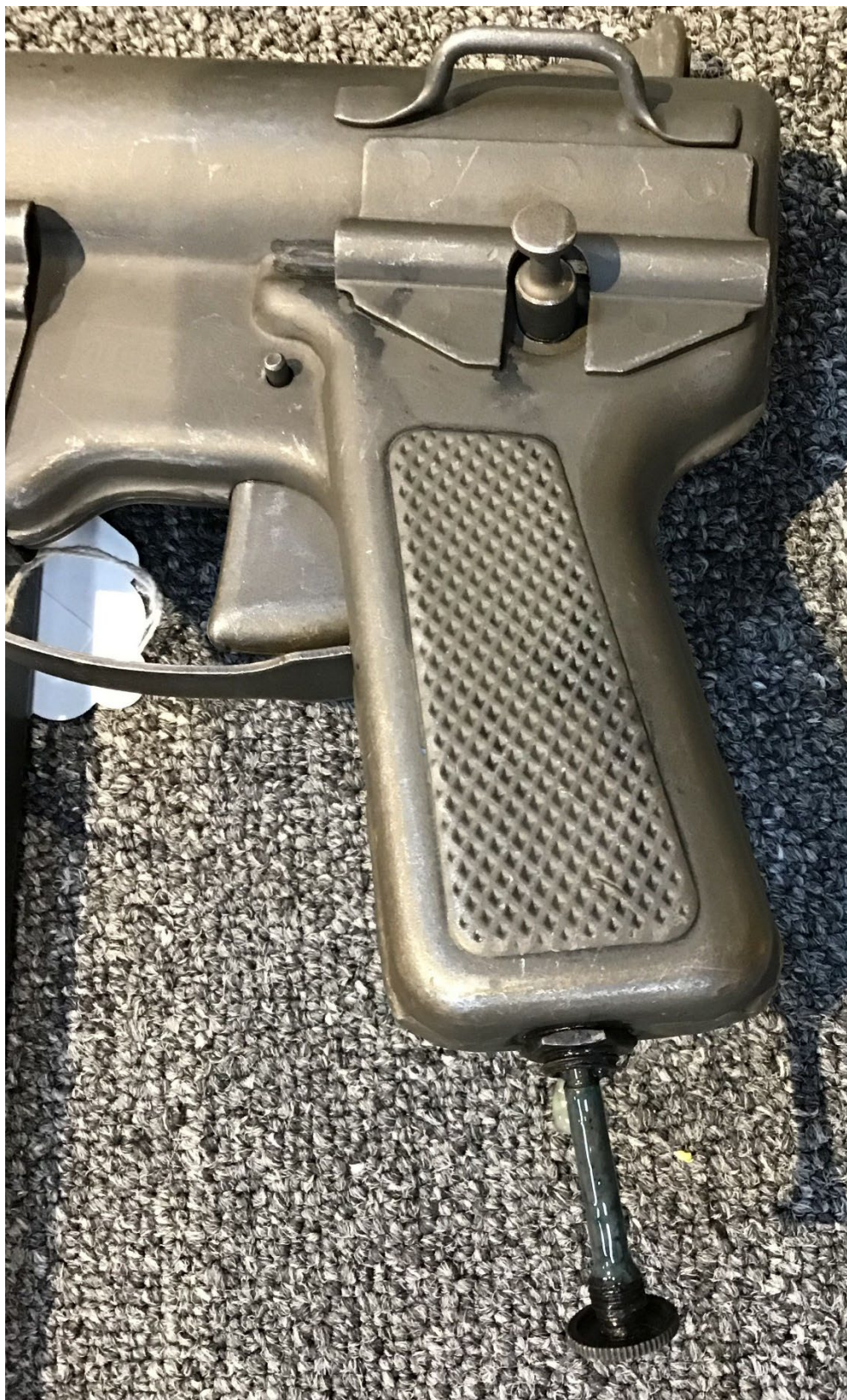
Sticking out of the pistol grip is the screw on oil brush partially removed. Inside is a compartment where oil is stored.
