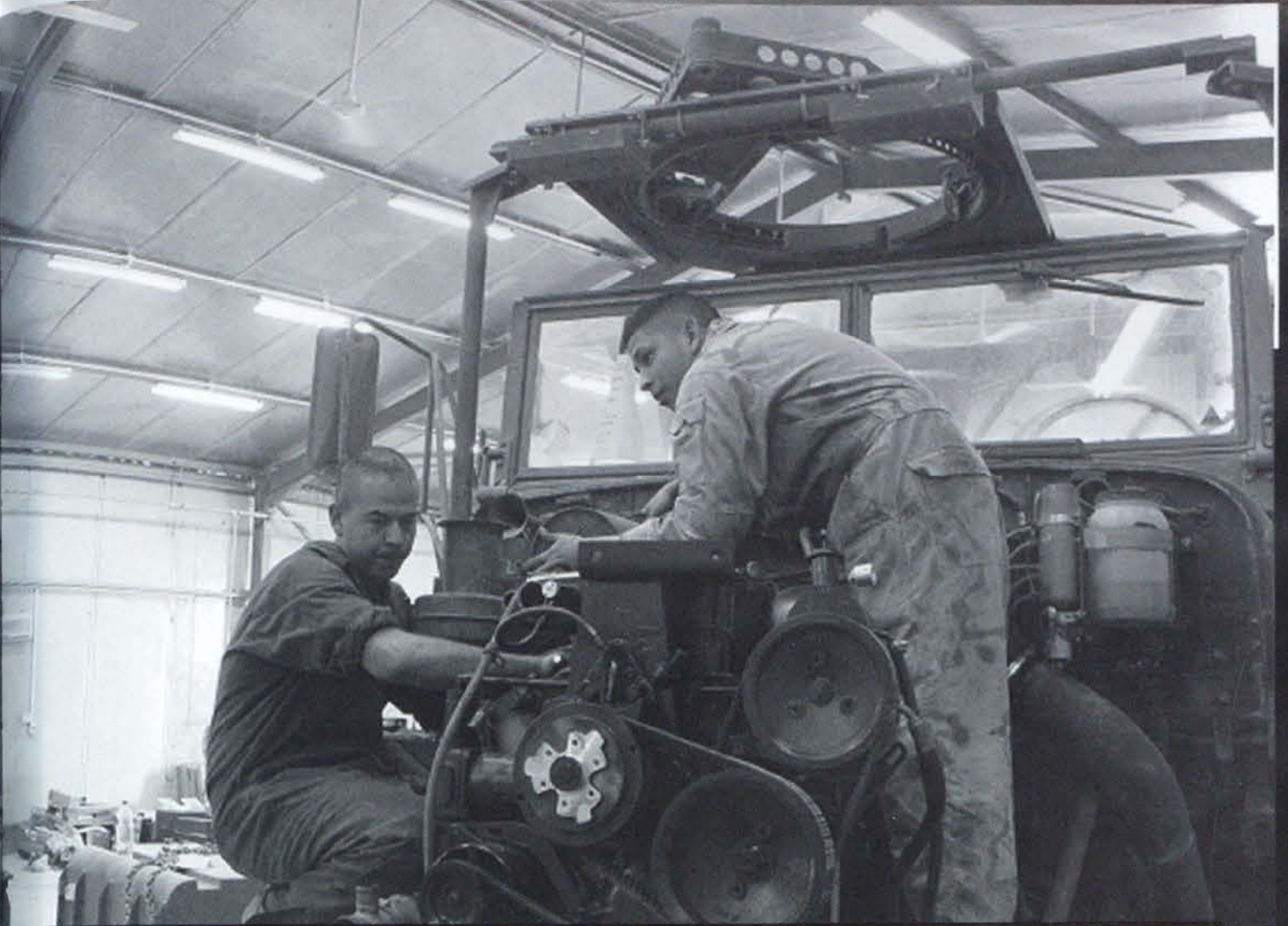
Above: SGT Larry Martinez and SGT Gabriel Rodriguez install an engine on a 5 ton truck. Below: SSG Ray Chavez and SPC John Lopez get there hands dirty with the wires in a HMWV.
